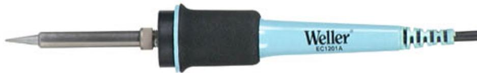
Weller standardized on the EC232 / TC218 style handle for many of its soldering irons in the early 1980s. This handle has been used for a variety of soldering irons and stations by Weller for the past 25 years.
